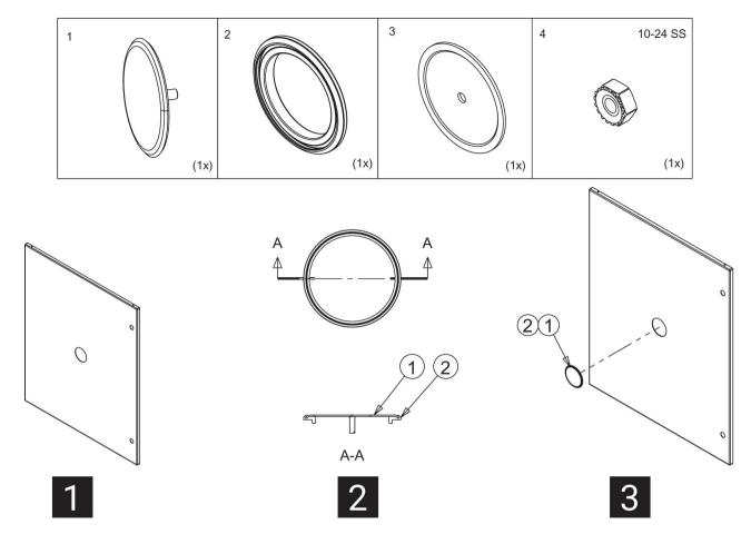
Check hole size in enclosure. See chart for hole diameter information. Clean and de-burr hole. Edge of hole should not be less than 12mm to the edge of the enclosure gland plate. Refer to cable gland instructions for minimum spacing of hole seals.
