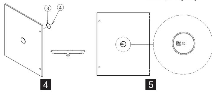
Mount retainer plate (item 3) on stud. Secure with hex nut (item 4) using 3/8 in. hex driver or wrench, torque to 18 in\*lb (2 N\*m). Do not over-tighten.
